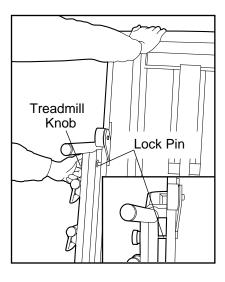
Slowly release the knob. Make sure that the lock pin is inserted into the hole in the treadmill frame.
